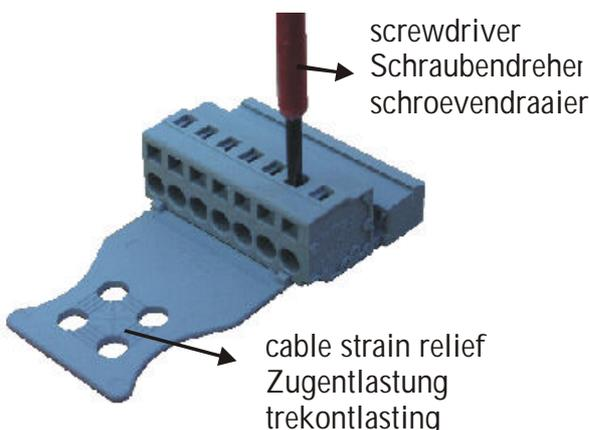
Open cage clamp by pushing the screwdriver.
